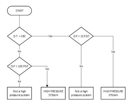
**Note:** Gas or fuel oil pressure piping systems covered in this code are those systems extending from the custody transfer point into a building or outside, above or below ground and where the design pressure exceeds the values in 1.1 a) or b) or c). Piping installations designed for a maximum pressure up to and including the values shown in 1.1 shall be
