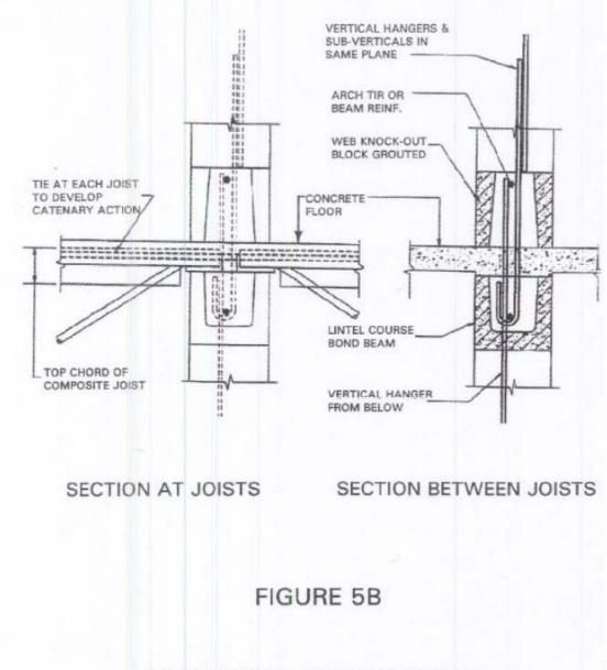
NOTE: AT EXTERIOR WALL, EXTEND JOIST BEARING BEYOND CENTRELINE OF LINTEL BOND BEAM AND TURN TIE BARS UP INTO WALL TO DEVELOP ANCHORAGE
