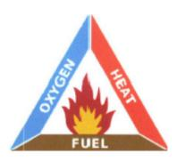
The fuel in this case is propane. In order to sustain a fire, all three components must be present. The use of internal valves and other pneumatically controlled equipment installed at the Breakaway Fuels site will severely restrict any fuel spills so the component of the triangle above will be severely curtailed.
