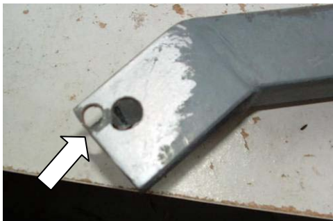
EXAMPLE OF ADDITIONAL HOLE TOO CLOSE TO EDGE (TOP VIEW)
