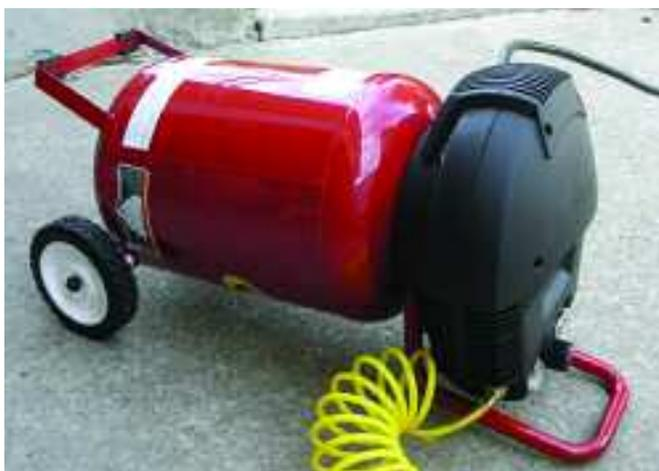
Standard CSA B51, *Boiler, Pressure Vessel and Pressure Piping Code* provide requirements for the proper design and construction of air receivers. Regulatory authorities adopt the Code across Canada as part of the pressure-equipment regulations governing the design, construction, operation and use of pressure vessels.
