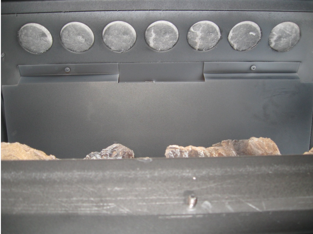
Pressure Relief Openings on Top of Firebox
